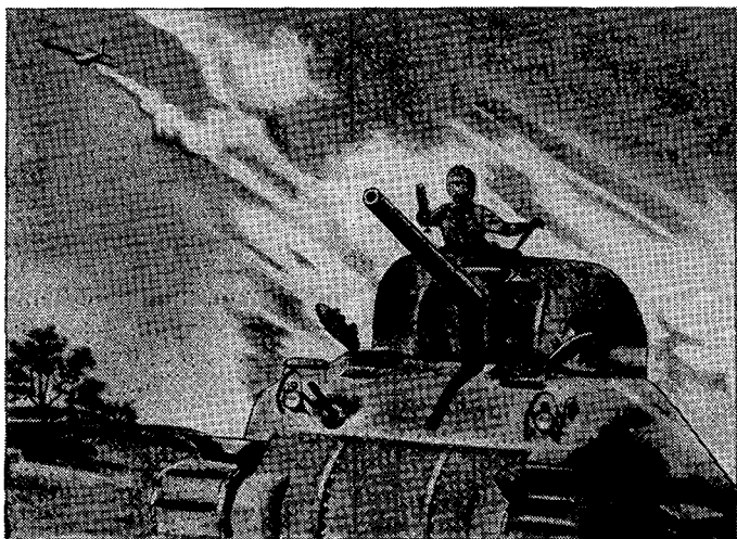
FIGURE 13.—Do not stop the tank as soon as it is contaminated. Continue until out of contaminated area. If you decontaminate while in the area, tank will be recontaminated from vegetation when you start.
